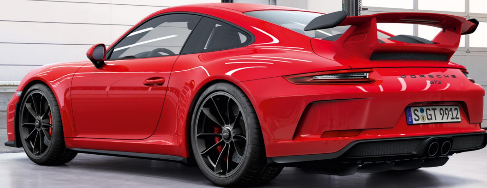
Squat is how the rear looks. And squat is also its stance on the road. That's because the 911 GT3 is an extra 44 mm wider and sits approximately 25 mm lower than the 911 Carrera. It's because the LED taillights are not only slimline, they are now also shaped three-dimensionally. It's because the central twin tailpipe of the sports exhaust system is a visual clue to the car's low centre of gravity.
